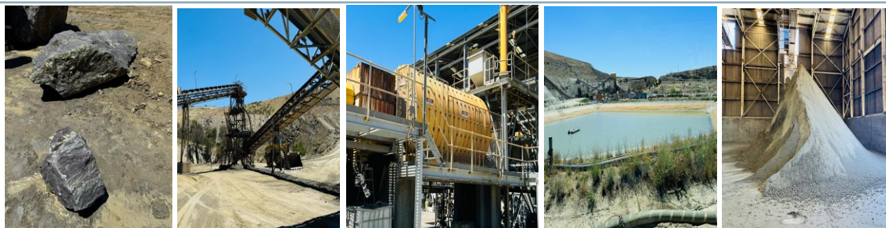
Figure 18. ROM ore, plant, TSF and 500t stockpile of concentrate
