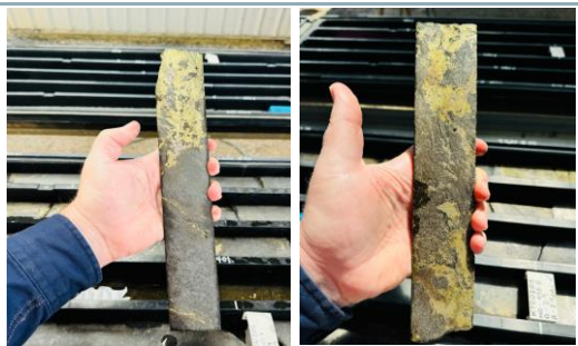
Figure 16. Drill core: Kavenagh's chalcopryite
